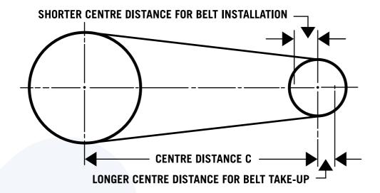
Note: Providing that the drive was designed correctly and that any adjusting slides and pivots are maintained, then there should be no problem fitting correct length belts.
