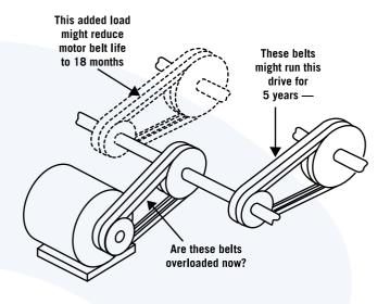
Added loads shorten belt life. A check should be made to see that no additional loads have been added since the original drive was selected. Take note of the drive system shown in the following illustration.
